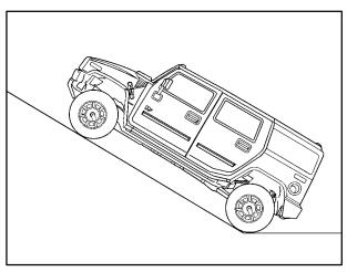
Also, specifications required that the HUMMER H2 be able to traverse a 40% ( $22^{\circ}$ ) side slope at 6 mph (9.7 km/h) while fully loaded on high friction surfaces.
